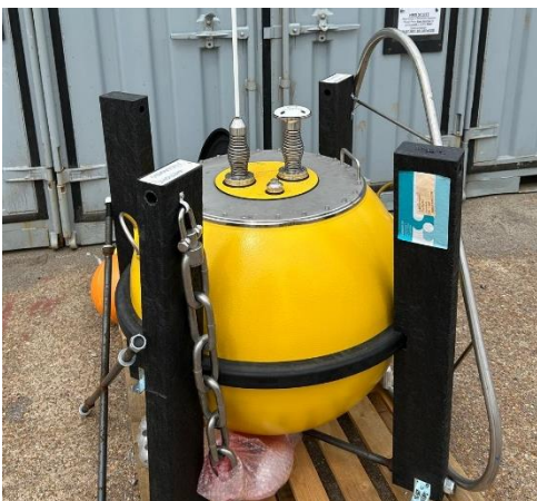
Photo on left of WaveRider buoy out of water and on right installed profile.
